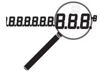
The Counter has 10 display digits to ensure that the display does not restrict the display resolution. It also has an overflow function that lets you see digit 11 and 12.
