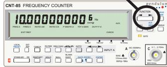
**FUNCTION** Press one end of the **FUNCTION** key. This scrolls the function cursor on the display. Release the key when the desired function is high-lighted.
