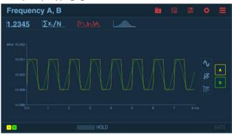
View fast FM, or any time/phase/frequency modulation, on screen, on one or two channels. Here we see FM modulation with both sine and square wave shape
