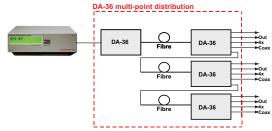
**Figure 3:** Multi-point distribution via cascading.
