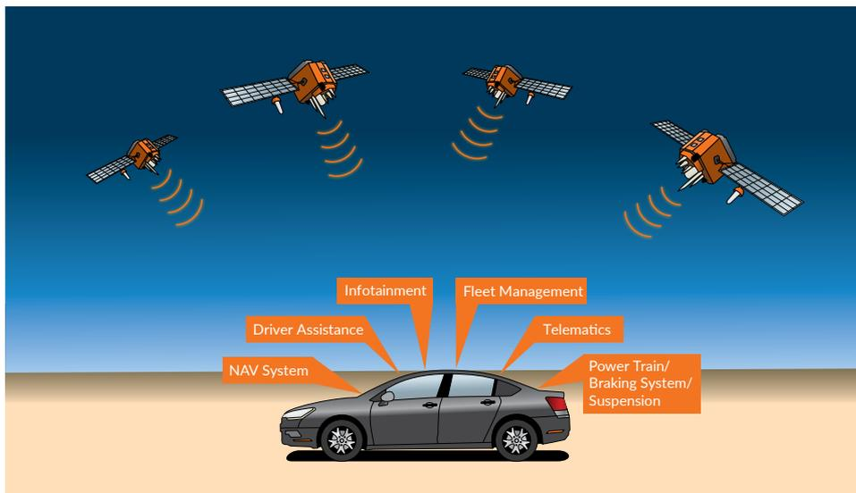
Automotive GPS subsystems are often limited to live-sky signals on the test track
