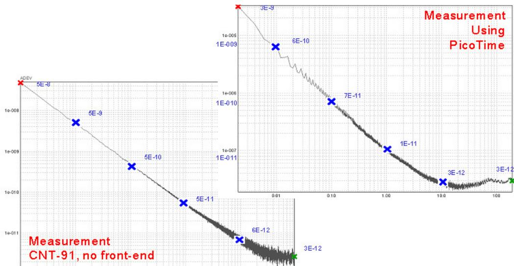
Figure 4. TimeView ADEV graphs of the same signal. One using CNT-91 + PicoTime and the other one only with the CNT-91
