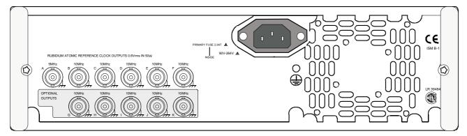
The frequency reference signals are available at the BNC-connectors on the rear panel. The rear panels of 6688 and 6689 are identical. This picture shows the 6689/021 version (11 BNC-outputs)
