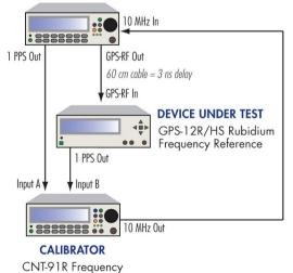
Figure 4. Measurement setup
