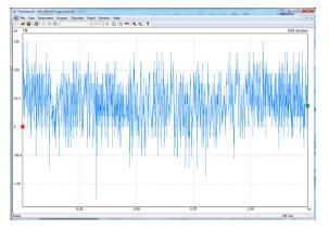
Figure 7. Stability of the reference 1 PPS output (TIE measurement)
