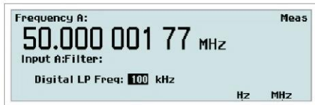
Fig. 3-7 Value input menu for setting the cutoff frequency of the digital filter.
