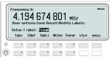
Fig. 2-35 Entering alphanumeric characters.
