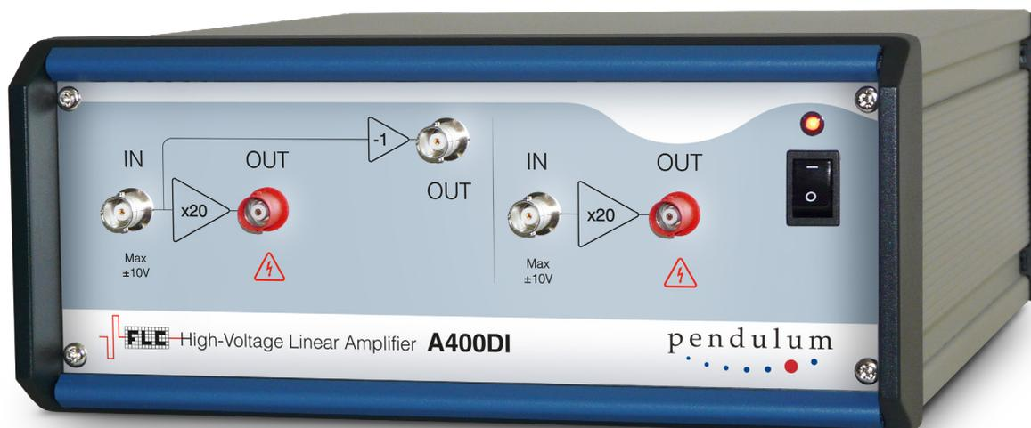
The Pendulum Instruments Dual Channel High Voltage Linear Amplifier A400DI contains two independent A400 amplifiers that share common ground reference and power supply. It features also a low voltage phase inverter that inverts the signal applied to the input of channel 1. The resulting signal can then be connected to the input of channel 2 by means of a short BNC cable (supplied).
