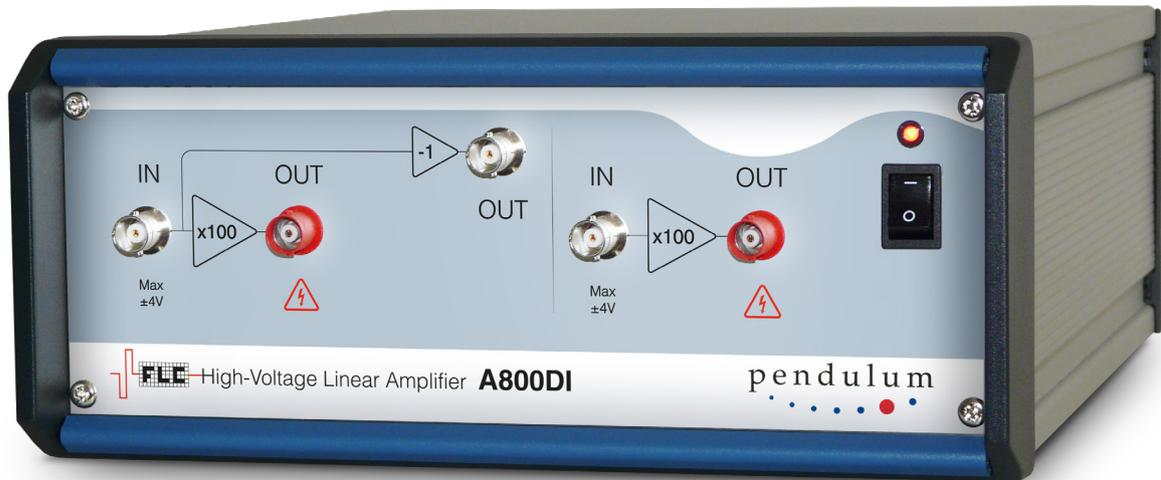
The Pendulum Instruments Dual Channel High Voltage Linear Amplifier A800DI contains two independent A800 amplifiers that share common ground reference and power supply. It features also a low voltage phase inverter that inverts the signal applied to the input of channel 1. The resulting signal can then be connected to the input of channel 2 by means of a short BNC cable (supplied).
