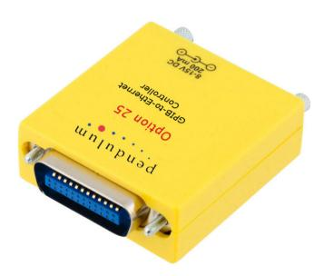
The Option 25, GPIB-to-Ethernet Controller, enables remote control and monitoring, of any Pendulum Counter/Analyzer in the CNT-90 series, over a LAN network. This new Ethernet control and monitoring interface, complements the two standard interfaces, GPIB and USB.
