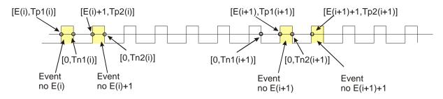
E(i) is the i:th sample of accumulated input cycles (ALL trigger events are counted and accumulated up to 160 MHz on input A or B,). E(i)=0 for the negative slopes, and the accumulated number of input cycles for the positive slope
