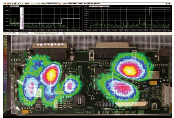
MultiScan measurement. The top left graph shows the accumulated trace (a max hold spectrum of all measuring points). The top right graph shows the wide band spectrum from a user selectable spot on the field plot.
