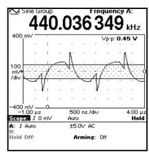
Figure 1. Waveform display showing trigger hysteresis band and level. There are no false counts even with the severe waveform distortion
