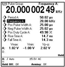
Figure 2. The pulse measurement group gives ten different measurements simultaneously.
