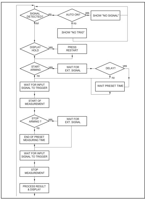
Fig. 7-5 Measurement control flow diagram.
