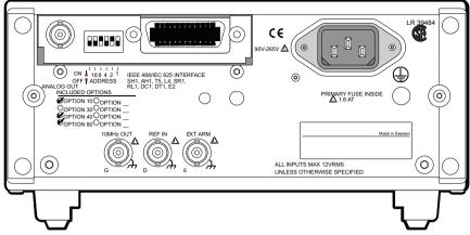
Fig. 3-2 Check marks on rear panel showing options included.
