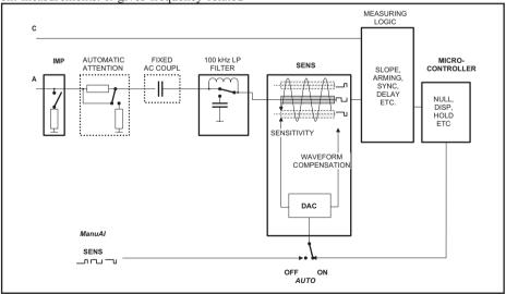
Fig. 5-1 CNT-85 Signal Conditioning Block Diagram.
