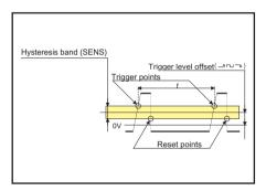
Fig. 6-13 Time is measured between the trigger point and the reset point.
