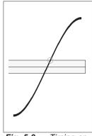
**Fig. 5-9** Timing error due to slew rate.
