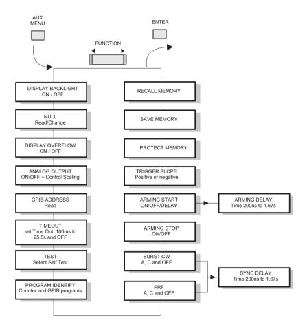
Fig. 9-1 You will enter the AUX MENU at the same selection as you used the previous time, except after power-on when you enter the menu at RE-CALL.
