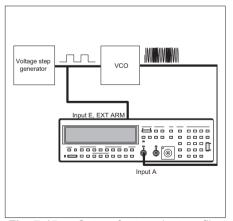
**Fig. 7-15** Set up for transient profiling of a VCO.
