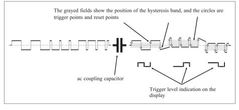
Fig. 5-3 Dc shift caused by the ac coupling capacitor.
