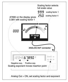
**Fig. 9-2** The analog output function.
