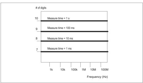
Fig. 1-1 Resolution of the counter.
