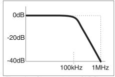
Fig. 5-4 Characteristics of LP filter.
