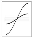
**Fig. 5-8** Low Amplitude delays the Trigger Point.
