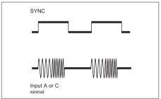
Fig. 7-12 A two-tone burst with its sync-pulse.
