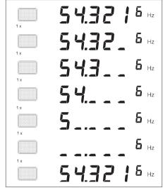
Fig. 7-1 Each press on the BLANK DIGITS key removes one diait.
