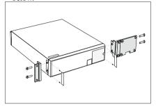
Fasten the CNT-85R in the rack via screws in the four rack-mounting holes
