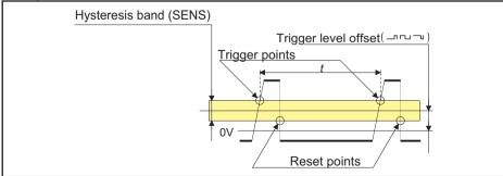
Parameters controlled by SENS and Waveform keys. Fig. 5-2
