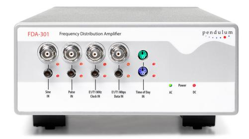
The Pendulum FDA-301 is a very versatile Frequency Distribution Amplifier for distributing a central time sync or frequency reference signal to multiple users, between rooms, floors, buildings and sites. The FDA-301 can distribute sine, pulse (e.g. 1-pps or IRIG DCLS), serial ToD and standard telecom signals, via noise-free optical fibers to up to 18 receivers, located up to 2 km away. The FDA-301 offers modularity, redundancy and ease-of-use.
