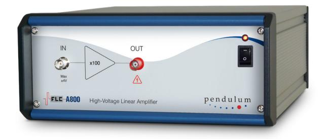
The Pendulum Instruments High Voltage Linear Amplifier A800 has a fixed amplification of 100 times and capable of bipolar high voltage output of  $\pm$ 400V. Any signal source with amplitude up to  $\pm$ 4 V can be used as an input device. The input amplitude should normally be kept within  $\pm$ 4 V. The A800 High Voltage Linear Amplifier is equipped with a microfuse rated at 40 mA, which will be blown if the input voltage exceeds 500% of the maximum.
