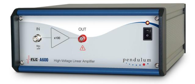
The Pendulum Instruments High Voltage Linear Amplifier A600 has a fixed amplification of 100 times and capable of bipolar high voltage output of  $\pm 300$ V. Any signal source with amplitude up to  $\pm 3$  V can be used as an input device. The input amplitude should normally be kept within  $\pm 3$  V. The A600 High Voltage Linear Amplifier is equipped with a microfuse rated at 40 mA, which will be blown if the input voltage exceeds 500% of the maximum.
