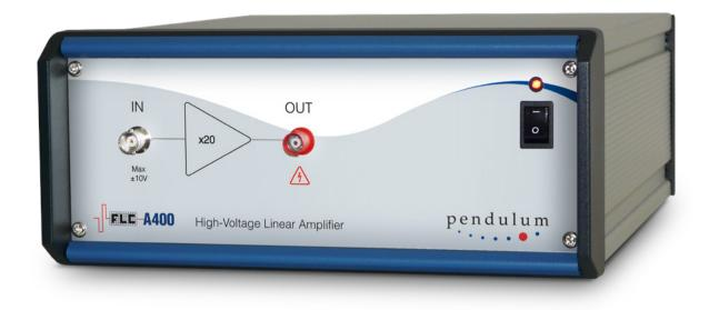
The Pendulum Instruments High Voltage Linear Amplifier A400 has a fixed amplification of 20 times and capable of bipolar high voltage output of  $\pm 200$ . Any other signal source with amplitude up to  $\pm 10$  V can be used as an input device. The A400 High Voltage Linear Amplifier is equipped with a microfuse rated at 40 mA, which will be blown if the input voltage exceeds 300% of the maximum.
